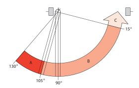
adjustment from fully open to 15 and 15 to closed.
