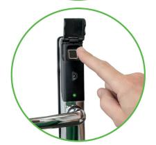
The third activation method is fingerprint recognition. A large fingerprint reading panel is concealed under a hinged cover on the external backplate. If you forget to lock the door, a 3 beep alert will remind you to do so.
