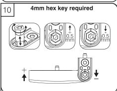
Compression adjustment: Push out hinge pin and turn to alter compression.
