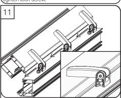
The sash can be removed and fitted when in an open position by lifting or lowering the sash assembly onto the frame datum.
