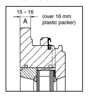
If dimension A (rebate height) is greater than 16 mm, the PVC packer supplied 2 must be installed below the locking hook.
