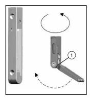
The MULTI Vent must be set to right or left so that Allen screw (1) can be accessed to set the braking effect.
